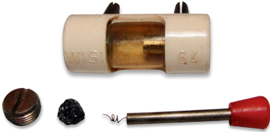
Plug-in crystal detector with pyrite crystal and spike
