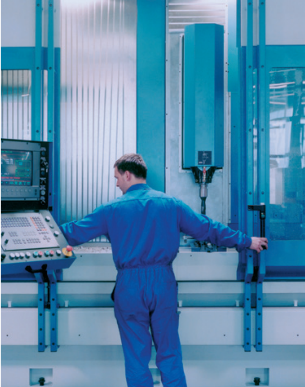
Example of the first applications of »energy harvesting« in industrial automation: A multifunction handle from the TGF programme on sliding doors eliminates the need for flexible cable systems.
