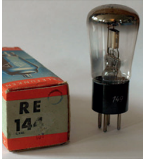
Tube type RE 144 of Telefunken (approx. 1920)
