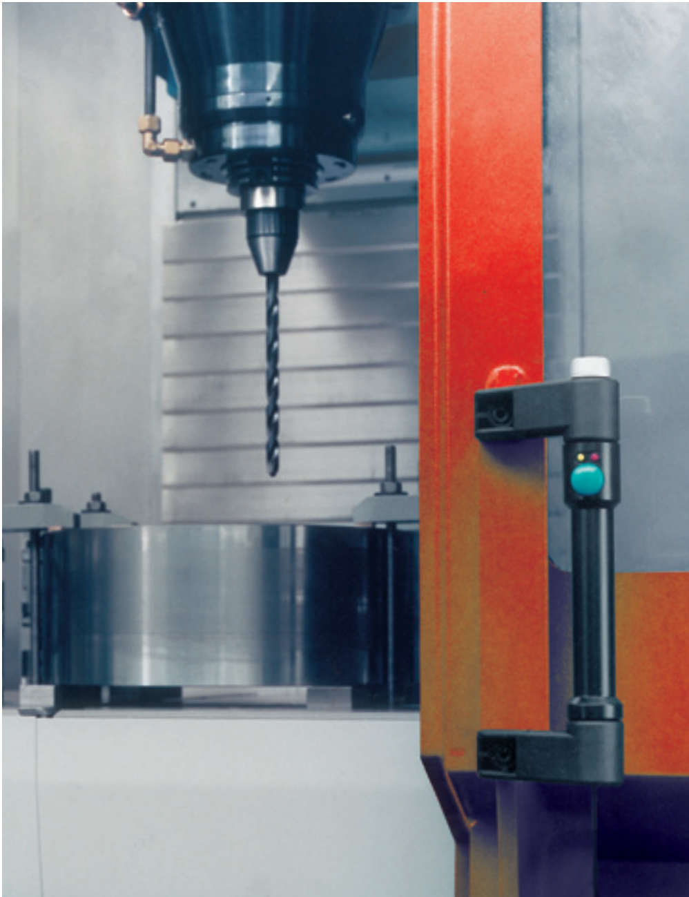
One of the first applications using EnOcean technology in industry: A wireless multifunction handle switch for machine tools.
