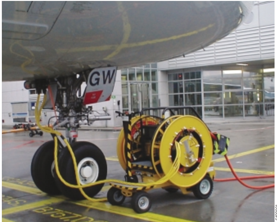
The Cavotec Caddy in action servicing an aircraft with 2x90k VA power.
