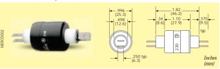
331 / 331 SS\* 3 conductor, 2x4 Amp. + 1x30 Amp. Disconnects included: 4 sm., 2 lg.
