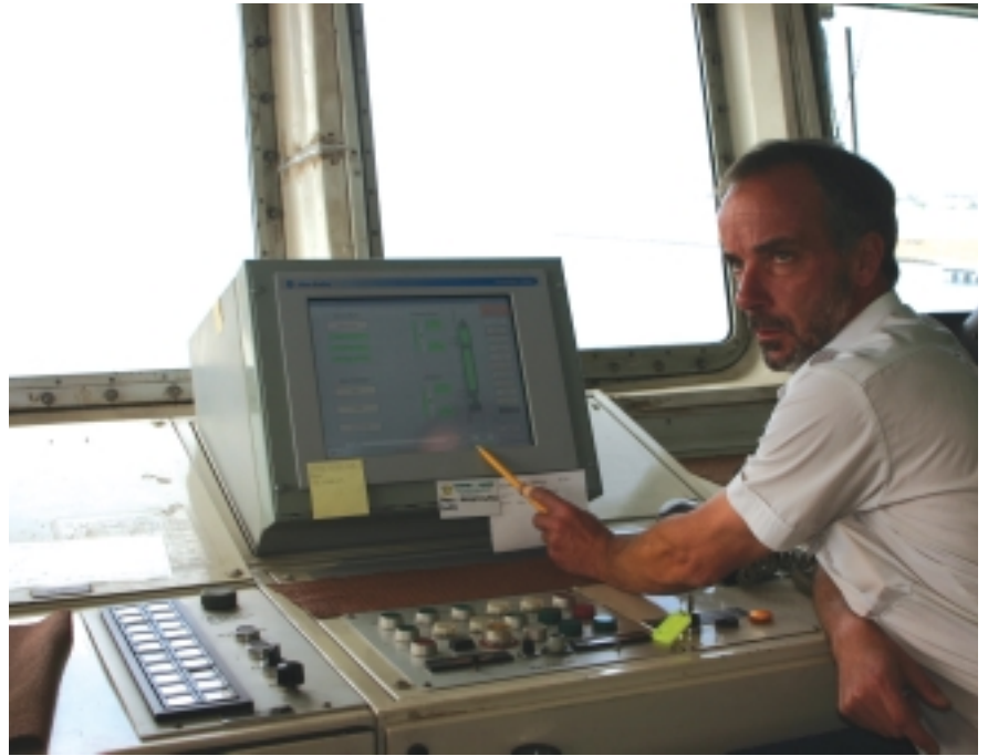
The system can be monitored and controlled in realtime directly from the bridge.
