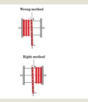
Figure 4. Winding of cable onto multi-spire reel.
