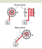
Figure 3. Transfer of cable from original delivery drum A to the cable winding reel B.
