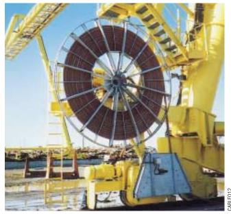
A Cavotec Specimas cable reel working at  $\pm 200 \text{ m/min}$  on a P&H log-handling crane for Federal Paper Board, in Augusta USA.
