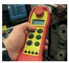
The MC-2-3 and MC-2-5 provide secure access through Pincode and access codes which restrict operation to a limited number of people.
