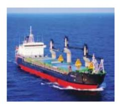
Today, most maritime cranes are operated by remote controls. This ship fitted with Mac Gregor cranes can be tandem operated increasing the maximum load that can be carried.
